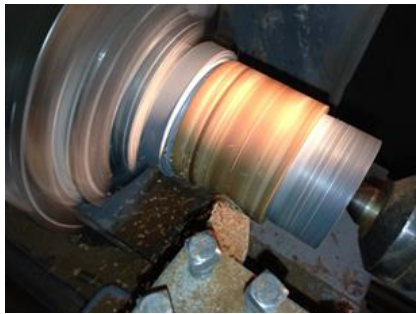
Sample manufacture by machine lathing
